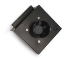
The AirShield is a separate accessory that can be purchased for any Microlab 600 instrument. It creates a positive pressure blanket of fresh air inside the pump that pushes air out over critical components on the outside of the pump, protecting them from the environment.
